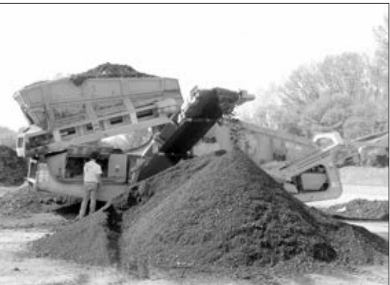
A large screener was brought onsite at the Waseca County Recycling Center last week to perform the final step before compost produced on site is ready for sale. Area residents can now purchase the material for use in gardens, raised beds, flower pots and landscaping at a price of $25 a ton or about one cent per pound. Amounts of material purchased at a time can range from bucketloads to trailers full. Pioneer photo by Deb Bently
